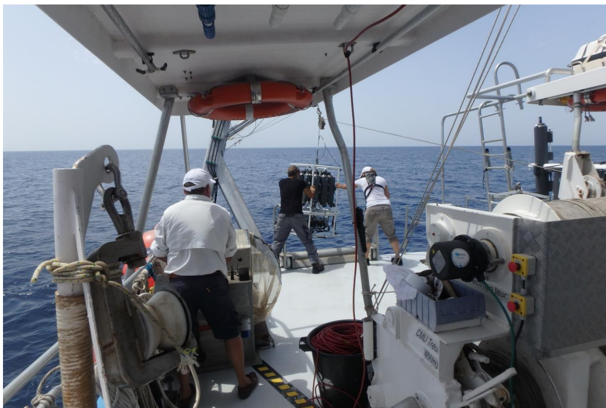
Deployment of the CTD Rosette at the BOUSSOLE site from the deck of the R/V Sagitta III
